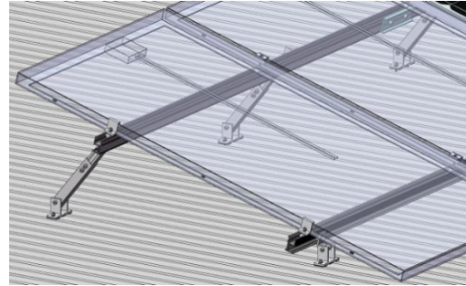
Install on tin roof directly
